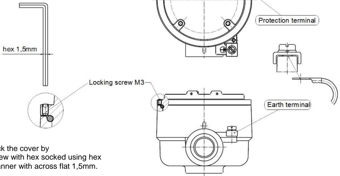
Lock the cover by screw with hex socketed using hex spanner with across flat 1,5mm.
