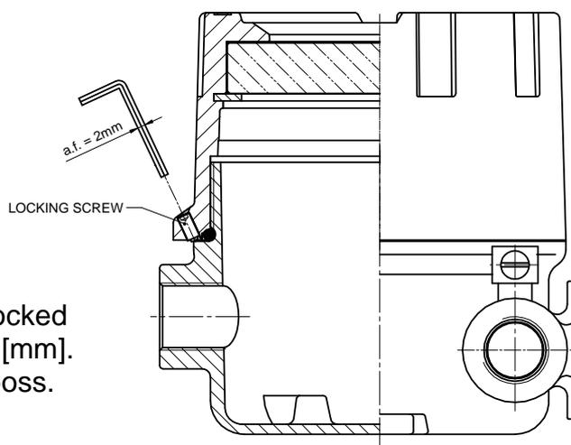
Cover is locked by screw with hex socketed using hex spanner with across flat 2 [mm]. This screw is situated on the cover boss.
